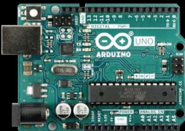
The FANCYSTICK is based on the ARDUINO UNO microcontroller patching. It has software and hardware components that ensure the interaction of the FANCYSTICK components allows control of electronic devices like a PlayStation.
